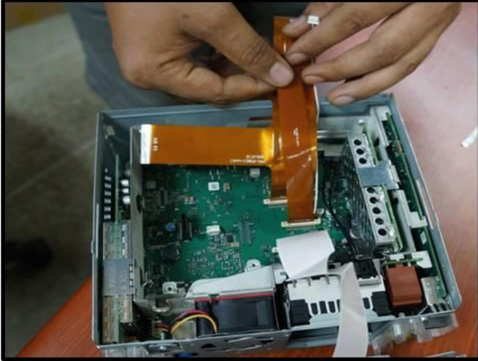
Key FPC cable connection
