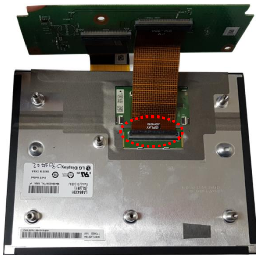
1. Disconnect the OEM FPC cable from the monitor
