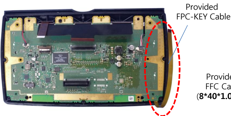
9. Assemble the monitor back again (FPC-KEY should be out from the monitor)
